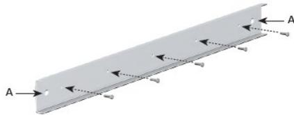
Figure 2: Drill cable entry (A) for connection cable in the mounting plate
