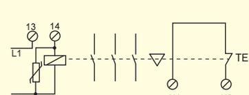
Control and supervision of external contactor, relay, valve or JOKAB SAFETY's expansion relays.
