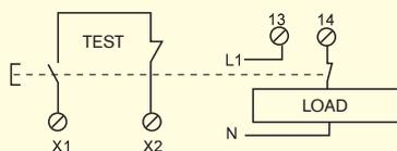
Monitoring to ensure that the Start button cannot stick in pressed position. Short circuiting over the closing contact is not monitored. The RT-series and JSBR4 have built in short circuiting monitored resetting.
