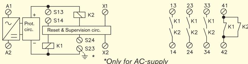
The electrical supply is connected across A1 and A2. After Voltage reduction and Rectification (AC-versions) or reverse polarity protection (DC-version) there is an overload protection-circuit.
