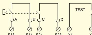
Enabling device, JSBD4. Stop condition is given in both top and bottom positions.
