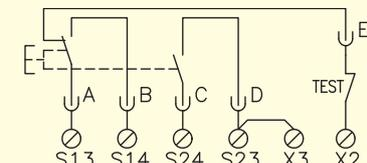
Enabling device, JSHD4. Stop condition is given in both top and bottom PB positions.
