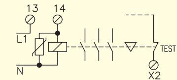
Control and supervision of external conductor, relay, valve or JOKAB SAFETY's expansion relays.
