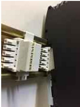
Fig. 1: DIN rail mounting with bus connector
