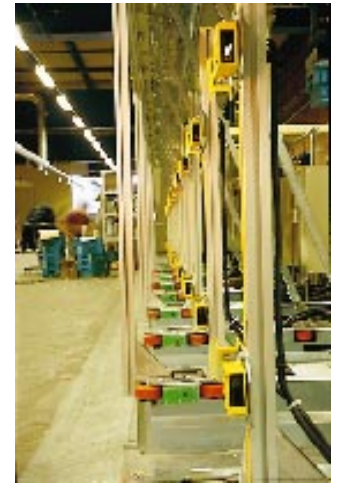
Light beams with automatic bypass at postal sorting depots in Gothenburg and Malmö.
